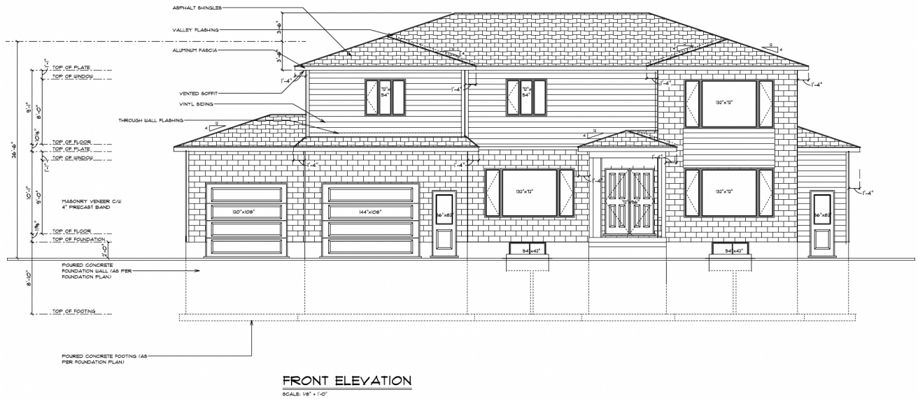
Figure 10: Front Elevation, prepared by Andre Theriault, April 30, 2024
