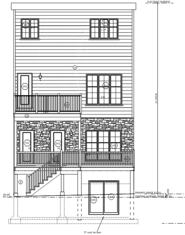
**Figure 6. Typical Side Elevation (3-Storey)**
