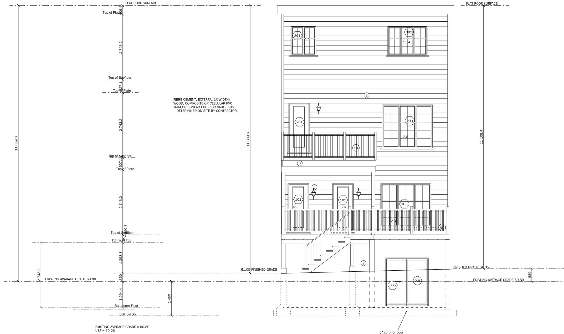
FIBRE CEMENT, EXTERRA, 1X(WIDTH) WOOD, COMPOSITE OR CELLULAR PVC TRIM OR SIMILAR EXTERIOR GRADE PANEL DETERMINED ON SITE BY CONTRACTOR.
