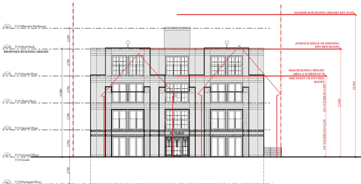
Figure 16: South Elevation showing proposed and existing massing and heights. Source: grc Architects 2021.
