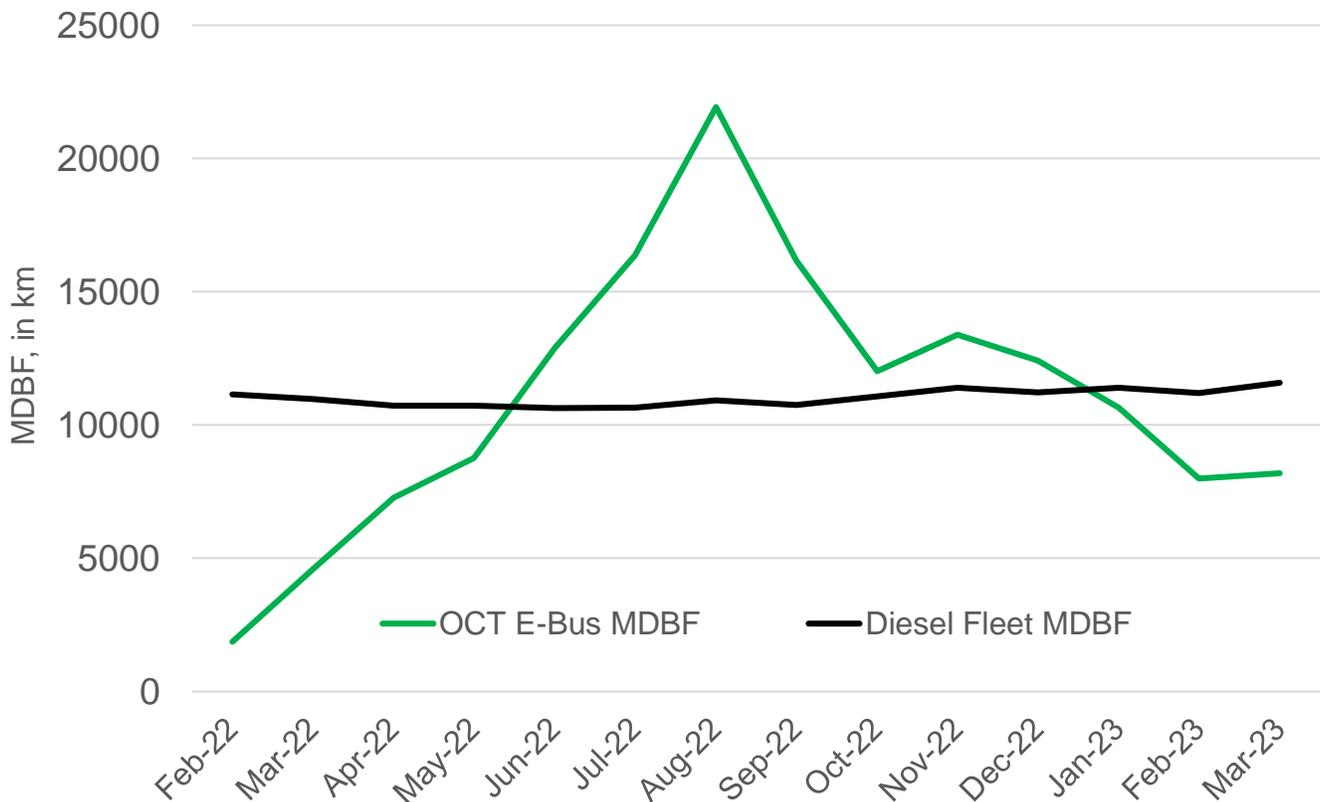
The E-Bus MDBF continued to climb as more kilometers were put on the fleet. However, with such a small sample size, any failures will result in a dramatic dip in the MDBF. The dip from
