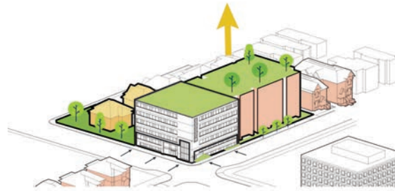
(3) Podium height references existing Legion building height and creates transition to the abutting neighbourhood - Elevate green space - Open ground floor of Legion to recreate a two-storey ground plane and increase site porosity
