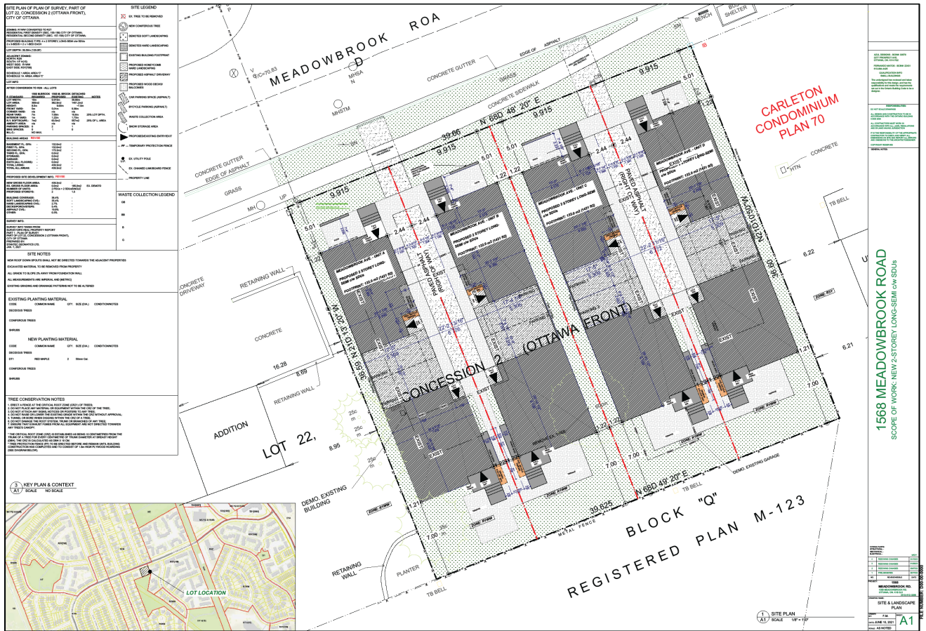
Figure 6: Proposed site concept showing four long semi-detached buildings. A PDF version of the concept plan is available on the Development Application Search Tool (Ottawa.ca/Devapps).
