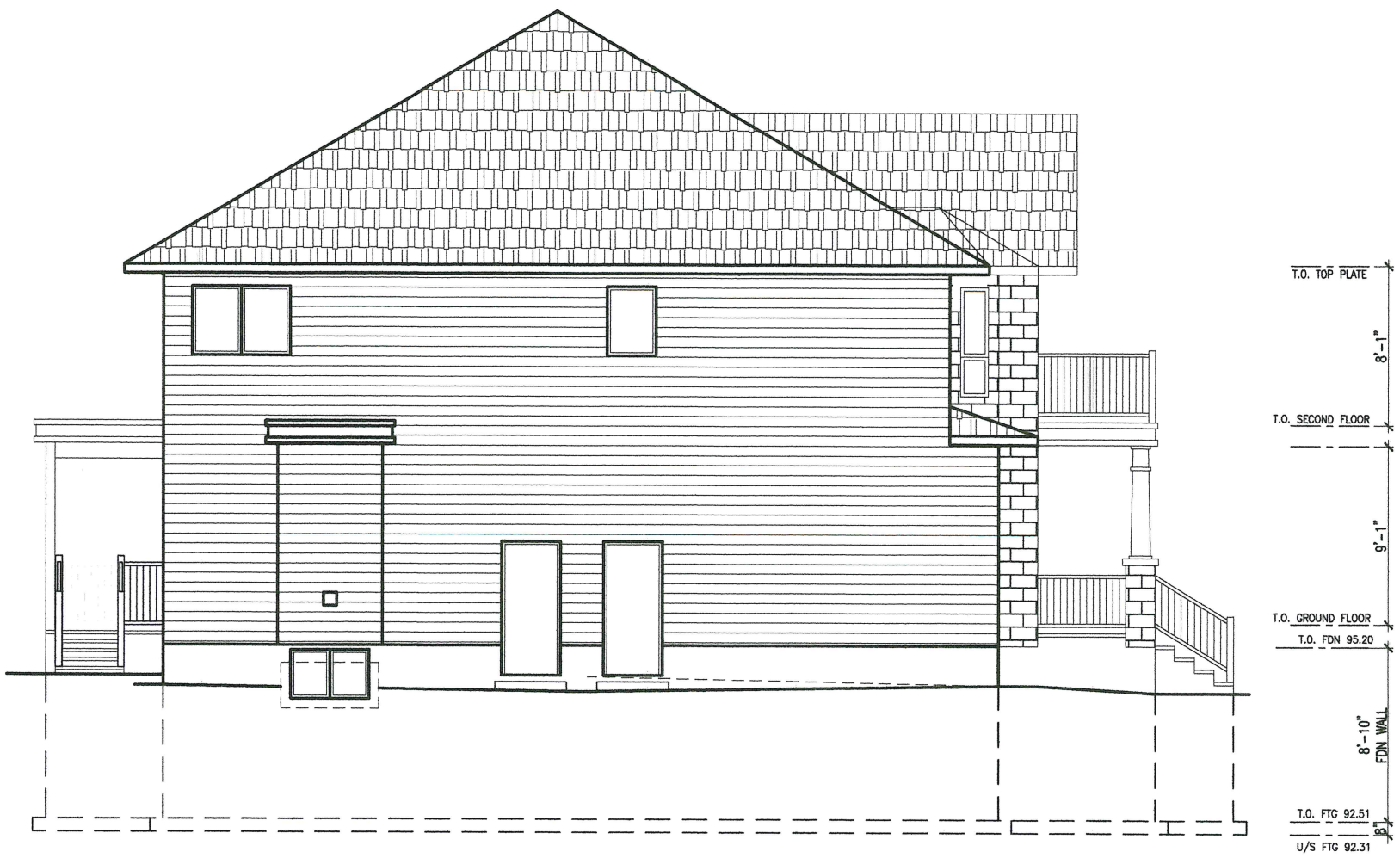
LEFT SIDE ELEVATION - PART 1 SCALE: 3/16" = 1'-0"
