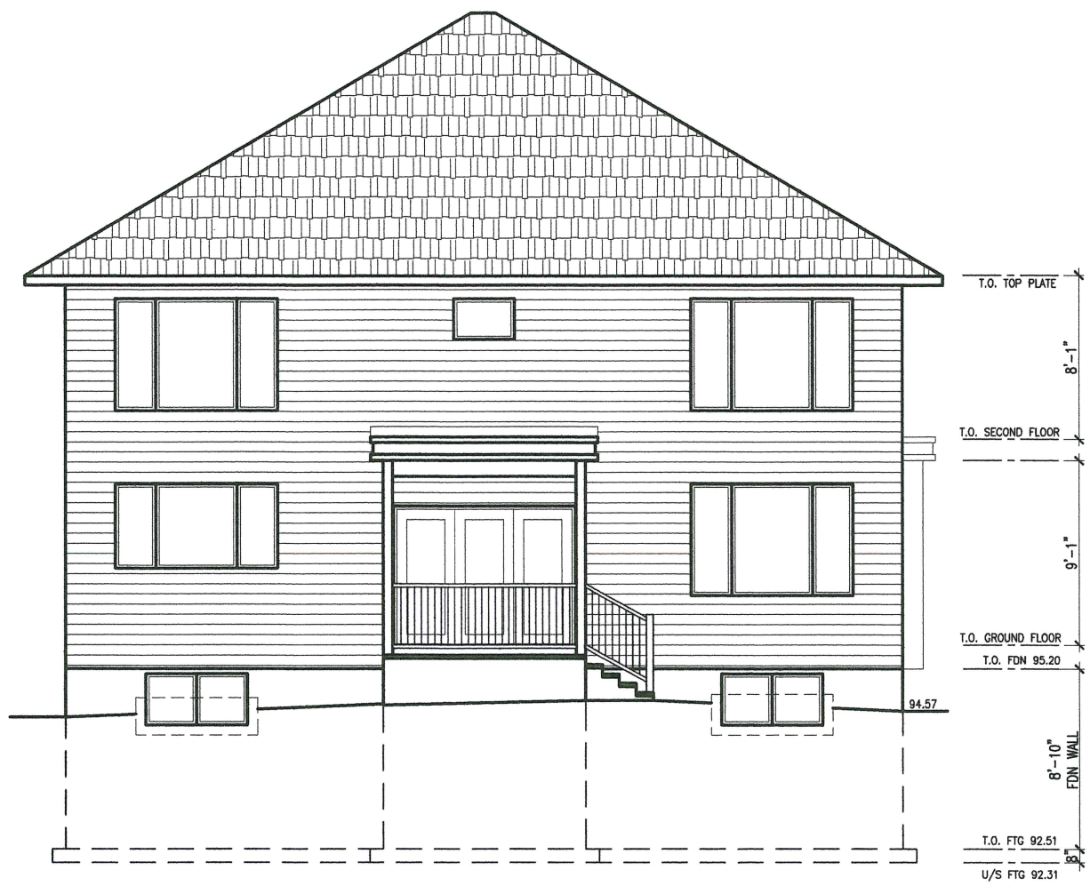
REAR ELEVATION - PART 2 SCALE: 3/16" = 1'-0"
