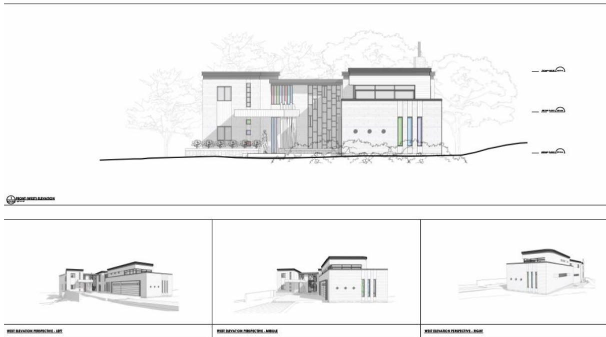
Figure 11: Views of the street elevation from various perspectives illustrating the relationship to the neighbouring property. The main entry is set well back from the street and the neighbour to the north with a 2-storey garage volume separated by the driveway. Native plantings have been proposed to flank the driveway and permeable paving is proposed for the driveway. A softer grey masonry façade is being illustrated. The side entry of the garage eliminates views from street of a gapping garage entrance. Source: Linebox Studio 2023.
