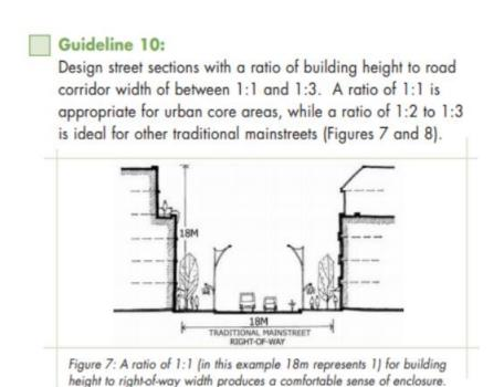
Figure 9 - Design Guidelines for Traditional Mainstreets Figure 7 illustrating step-back's above the 4th floor. (City of Ottawa)
