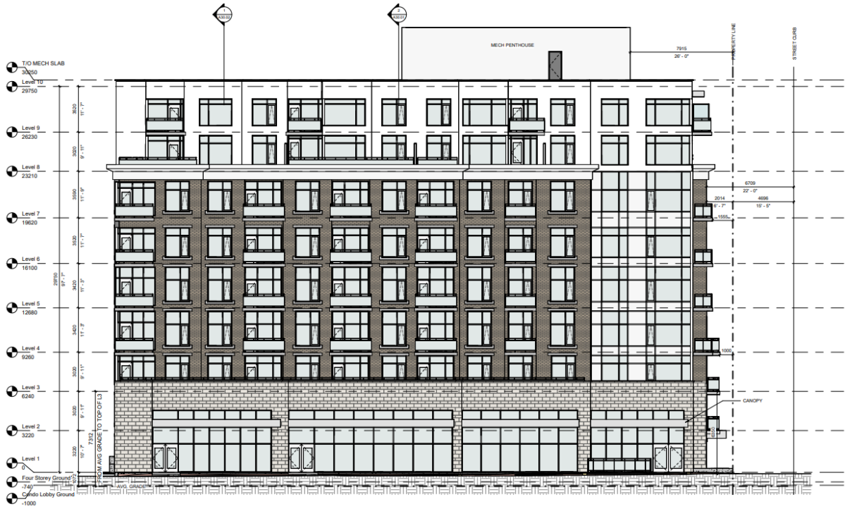
1 SOUTH BUILDING ELEVATION 1:100
