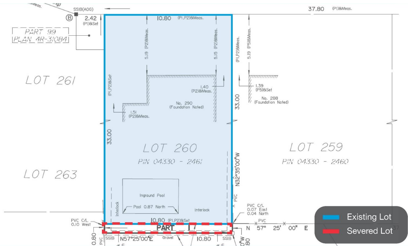
Figure 3: Colour overlay on the draft M-plan showing the existing lot of 290 Mount Nebo Way in blue and the part of lot from 316 Memorial Grove to be severed in red.
