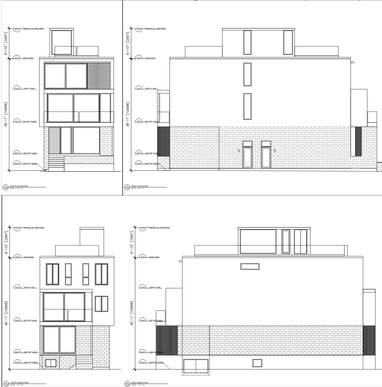
Figure 6: Elevations for the Proposed Development
