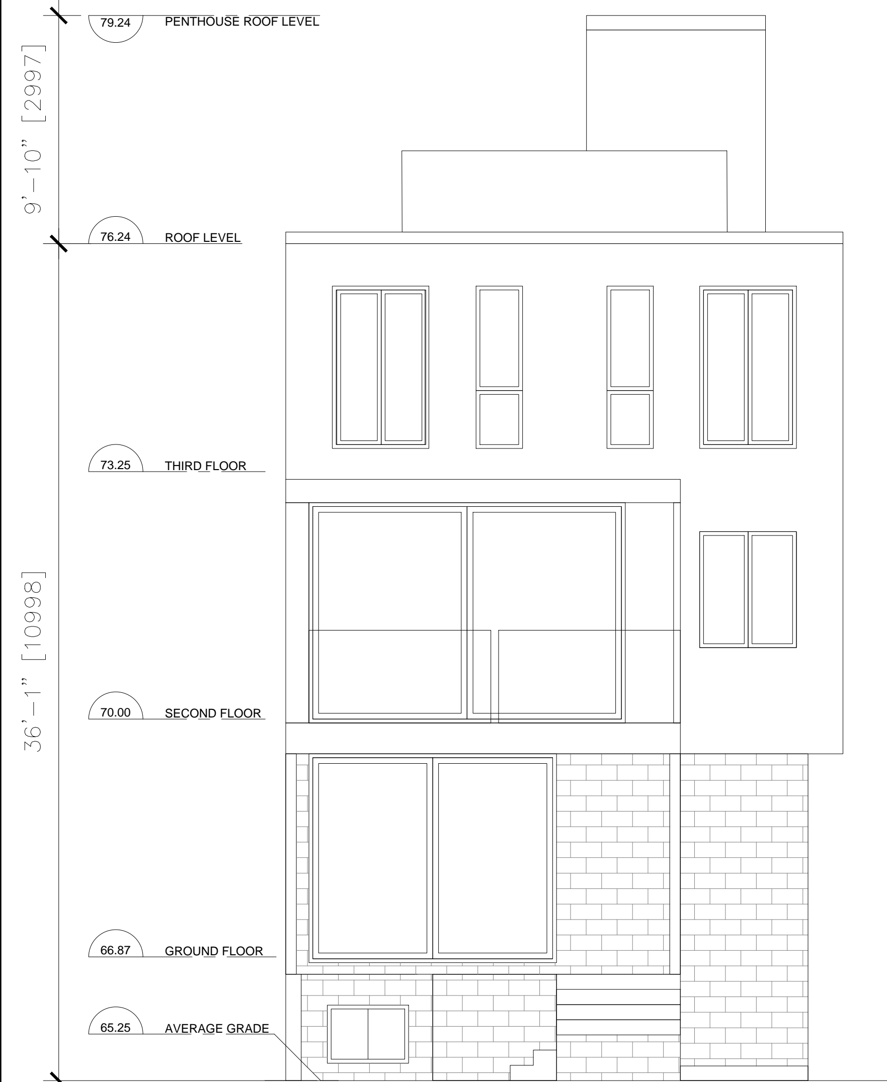
03 NORTH ELEVATION SCALE 1/4" = 1'-0"
