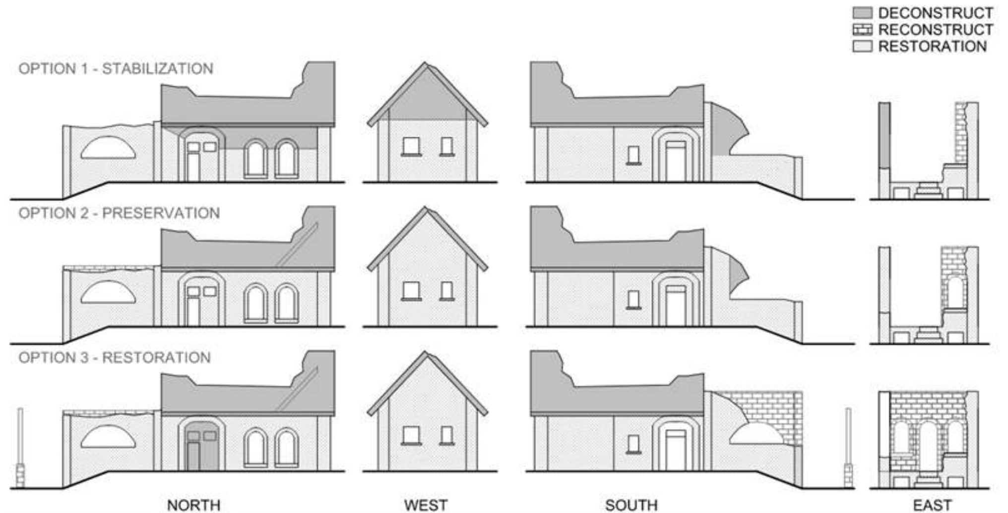
Image 1.9 Illustrations of stabilization options - Source: J.G. Cooke, 2021
