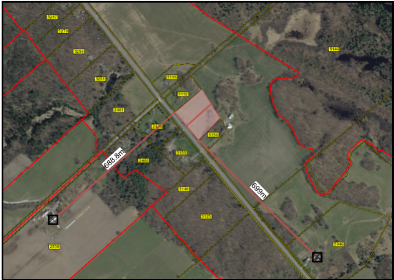
Image showing the subject properties to be severed and their distances to livestock barns within a 750m radius.
