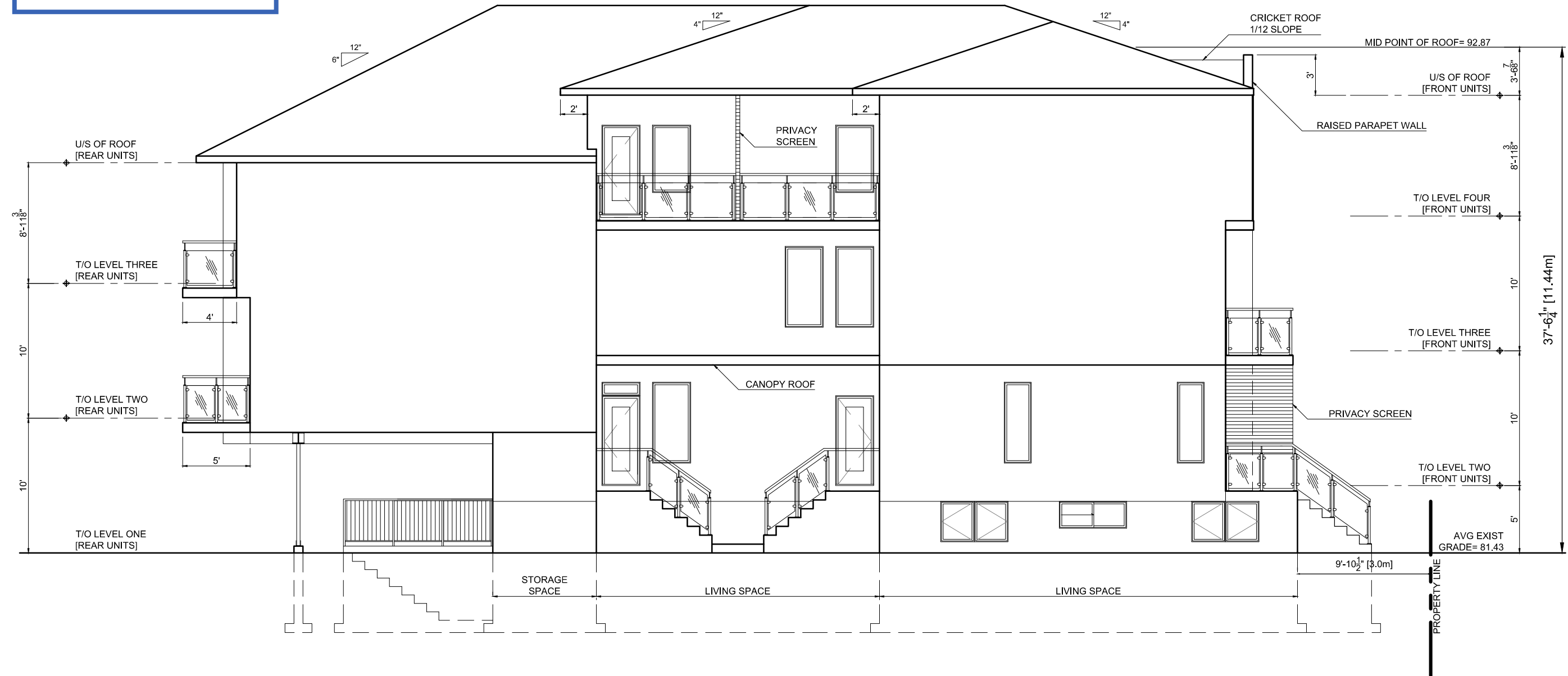
SIDE ELEVATION 2 [WALKWAY SIDE] SCALE: 1/8"=1'-0"
