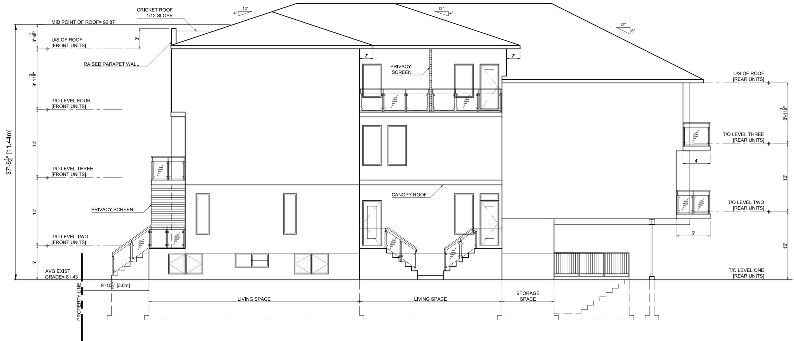
SIDE ELEVATION 1 [WALKWAY SIDE] SCALE: 1/8"=1'-0"
