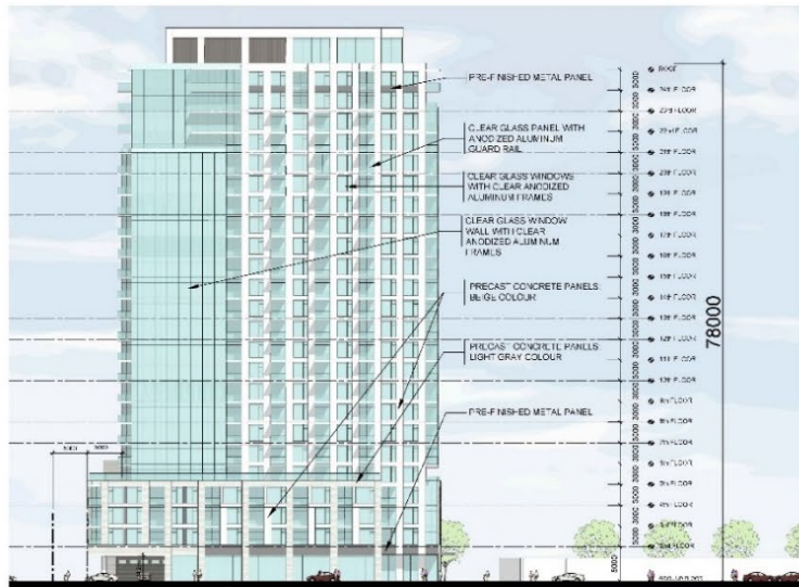
03 EAST ELEVATION BUILDING A
