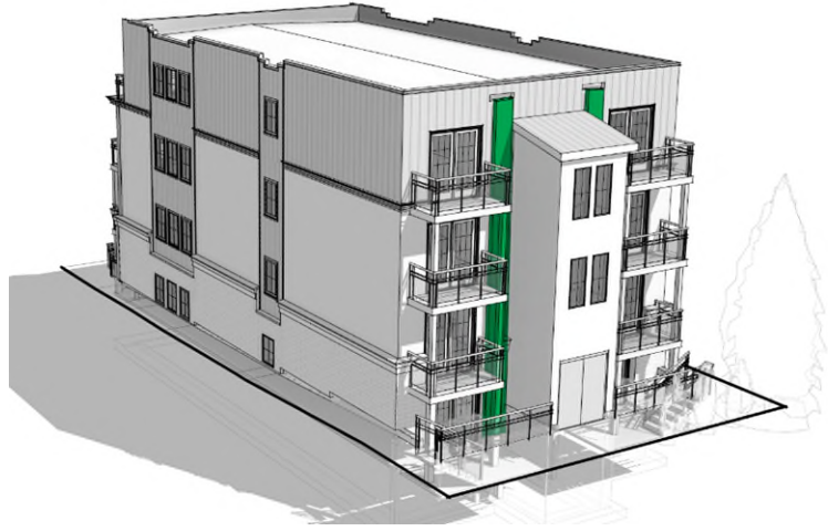
Figure 7: 82 Genest Street as seen from the South. The green high lights indicate the thru-wall scupper drains which connect to the building's weeping tile, VADD 2023.
