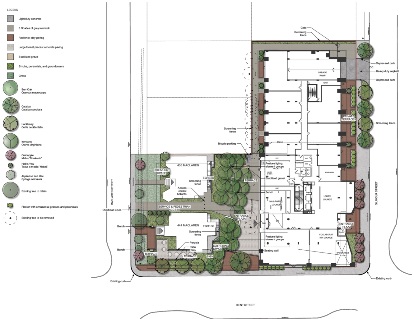
Figure 15: Site/landscape plan illustrating the relationship of the proposed development to the street and the two heritage buildings at 444 and 436 MacLaren Street. Source: Lashley & Associates Landscape Architects July 2023.
