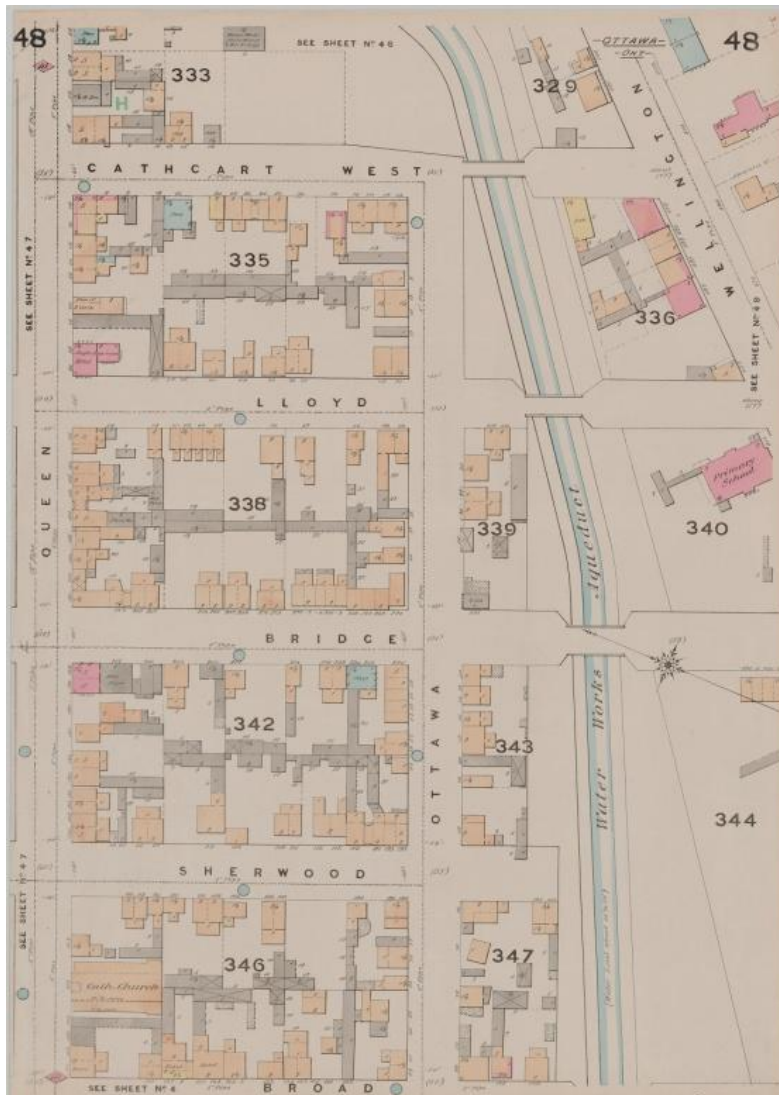
Figure 19: Fire Insurance Plan, 1878, detail showing the Old Booth Street Bridge. The bridge is depicted as being about half the width of the street, with is 61 feet (15.75 m) wide. Source: Library and Archives Canada, e010695525 sheet 48.
