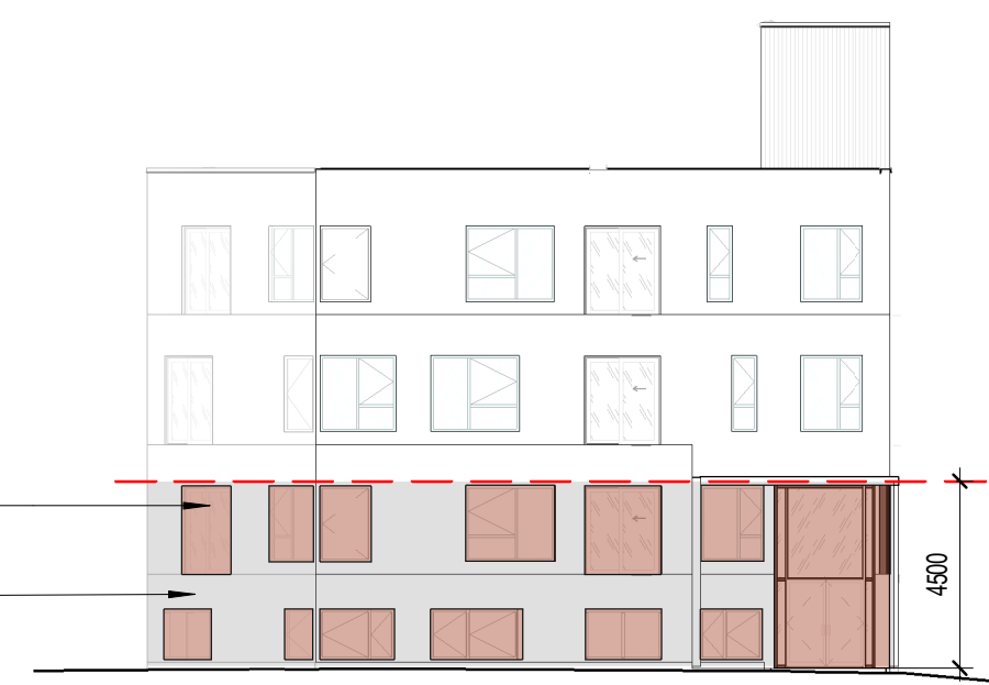
SOUTH ELEVATION - GLAZING REQUIREMENT ON CARLING 1 : 200
