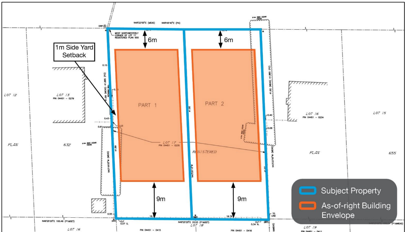
Figure 3: As-of-right building footprint of the retained and severed parcels
