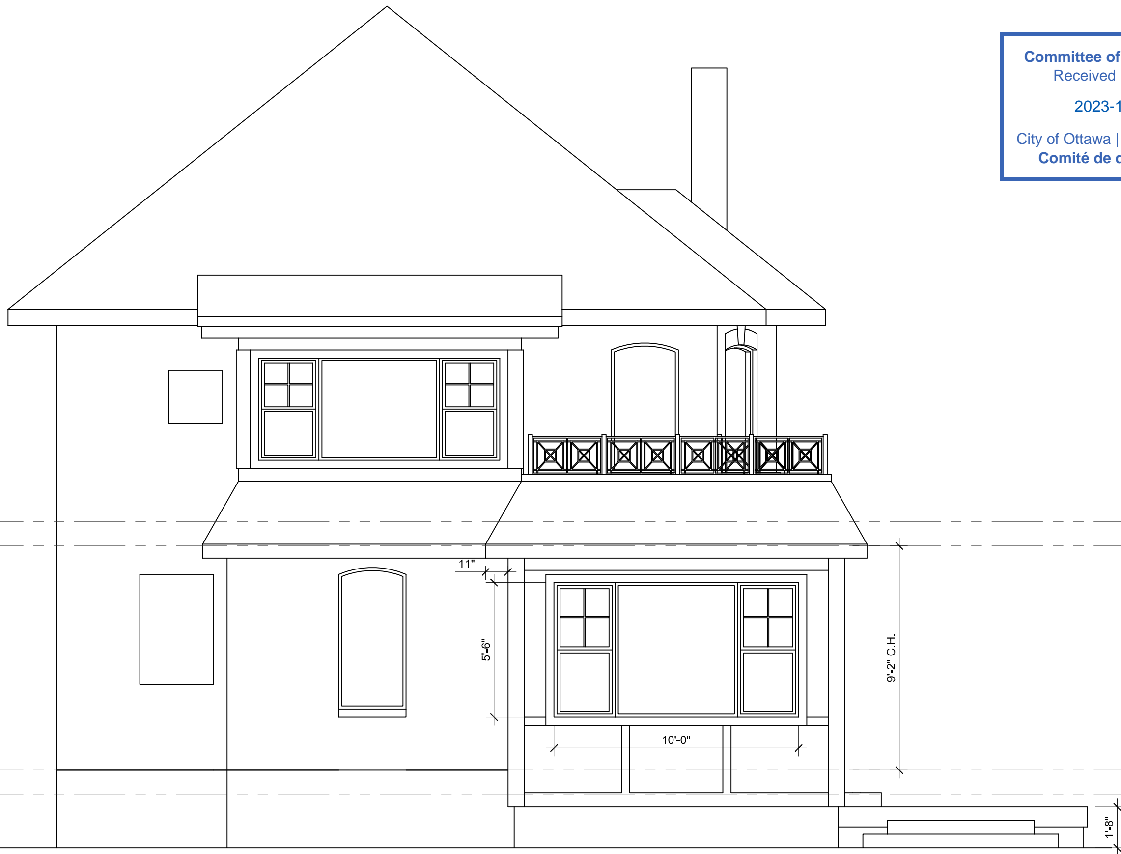
01 PROPOSED REAR ELEVATION ID1.5 1/4"=1'-0"
