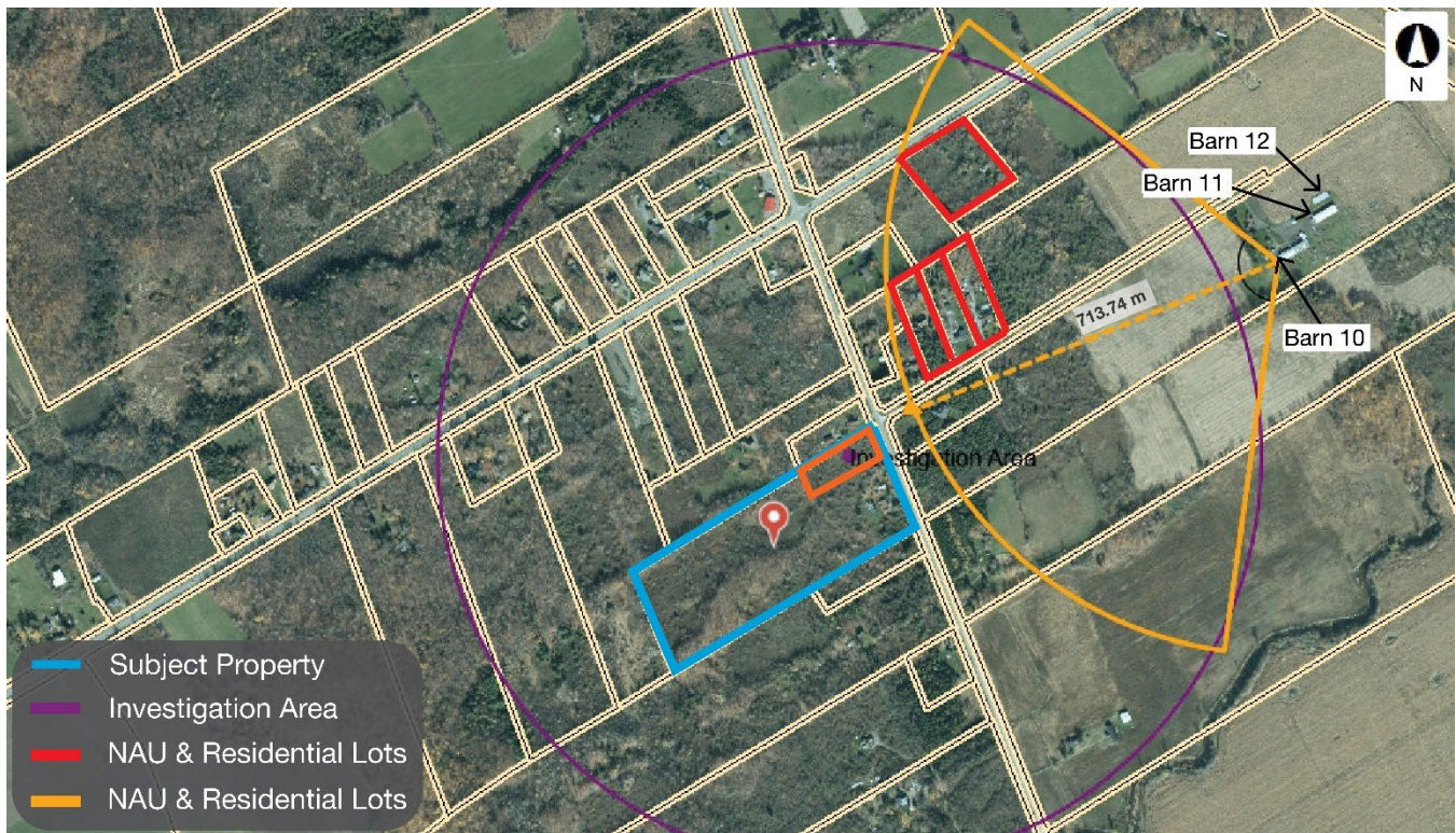
Figure 12. Application of IG #12 for Barn 10, 11 and 12 at 9158 McKeown Farm Road demonstrating non-agricultural uses (NAU) and residential uses within the 120-degree intervening area
