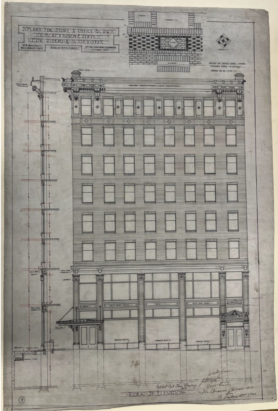
W.E. Noffke's original 1913 drawing of the Rideau Street elevation for the Plaza Building. 7
