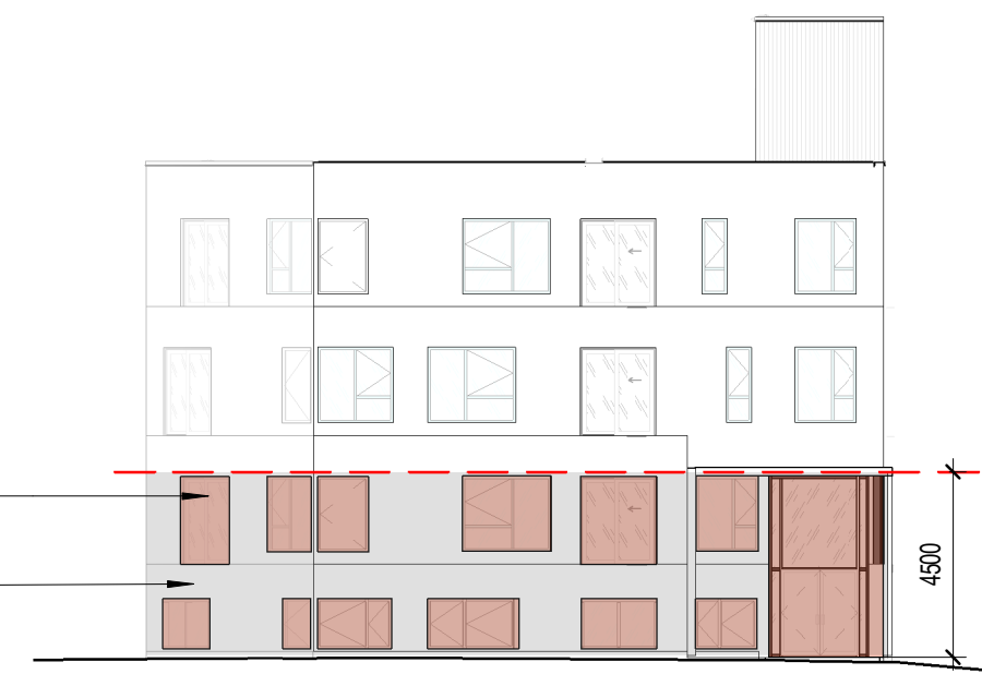
SOUTH ELEVATION - GLAZING REQUIREMENT ON CARLING 1 : 200
