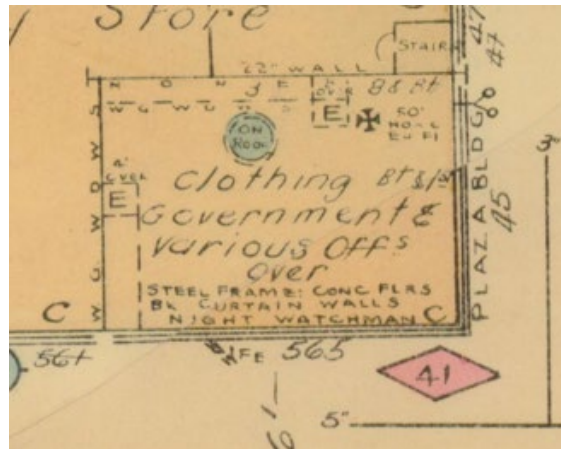
The Plaza Building on the 1948 Fire Insurance Plan indicating that it is a steel frame
