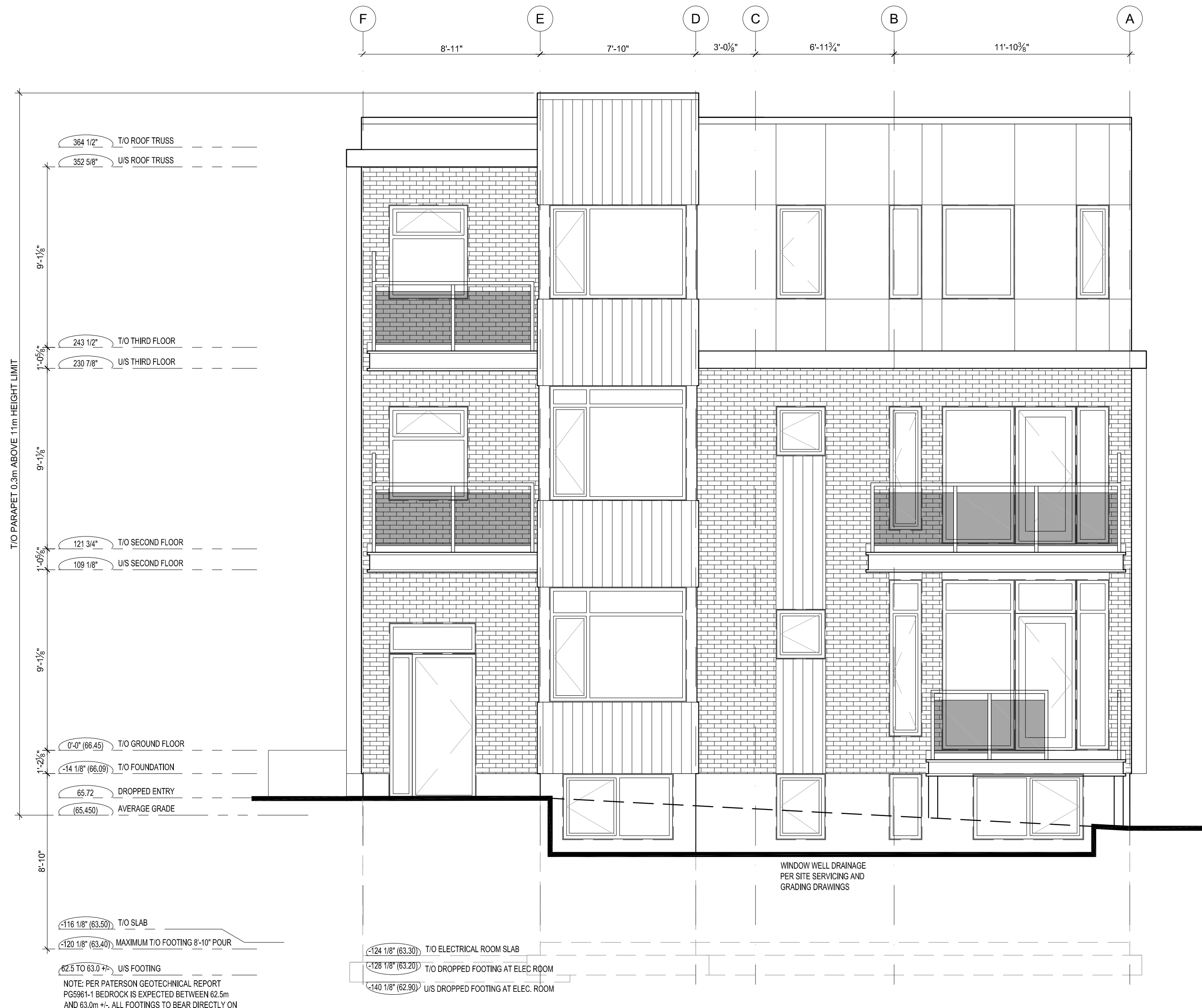
1 FRONT ELEVATION A2.1 SCALE: 1/4"=1'-0"
