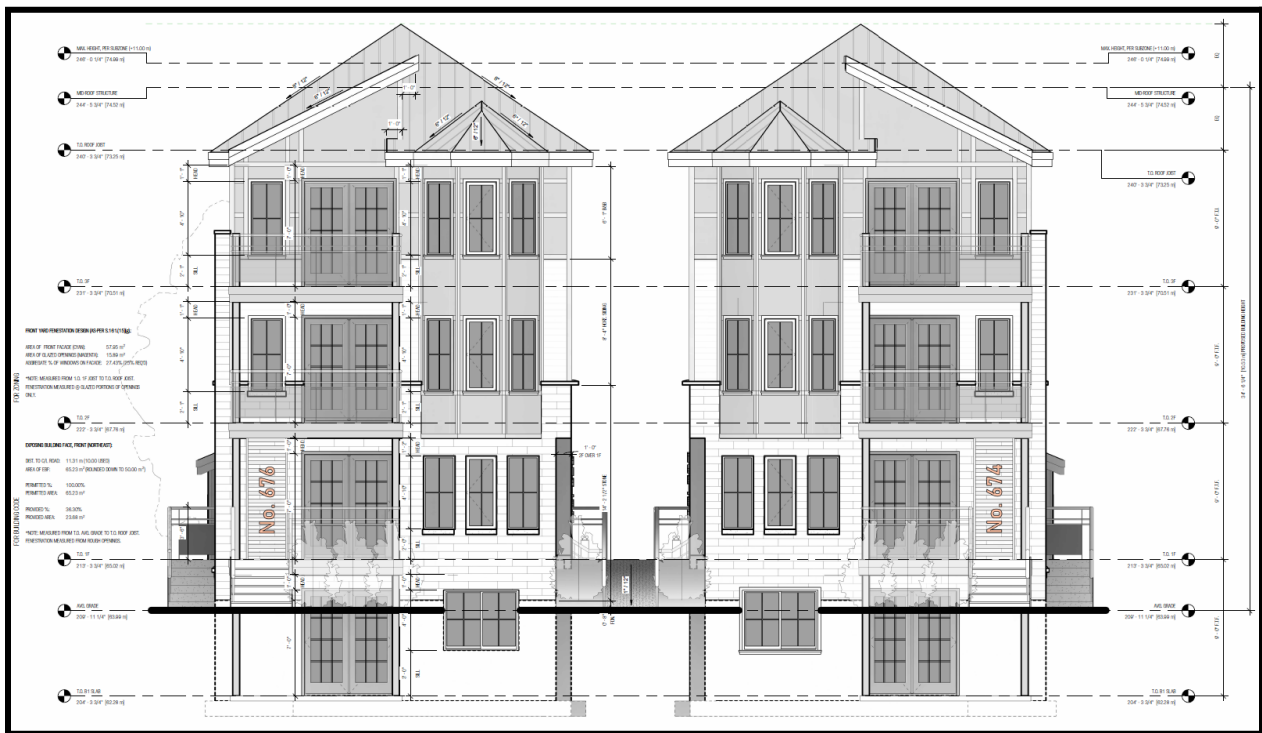
Elevation on De l'Église St (east) demonstrating the area of windows compared to the facade area.
