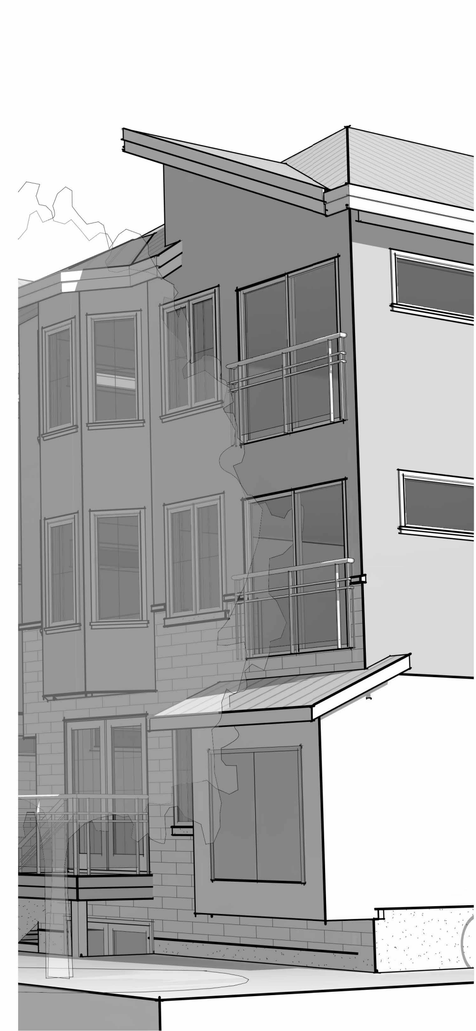
REGIS AVENUE APPROACH: NOTE THE ELEVATED HYDRO ENCLOSURE & JULIETTE BALCONIES
