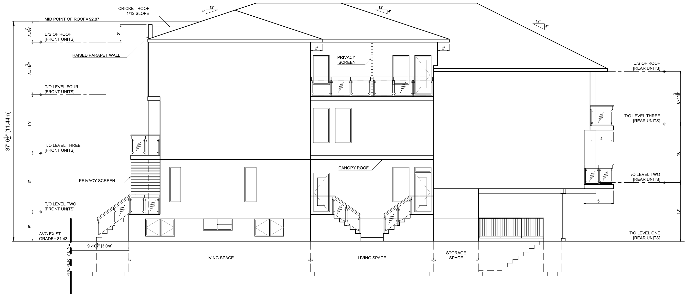
SIDE ELEVATION 1 [WALKWAY SIDE] SCALE: 1/8"=1'-0"
