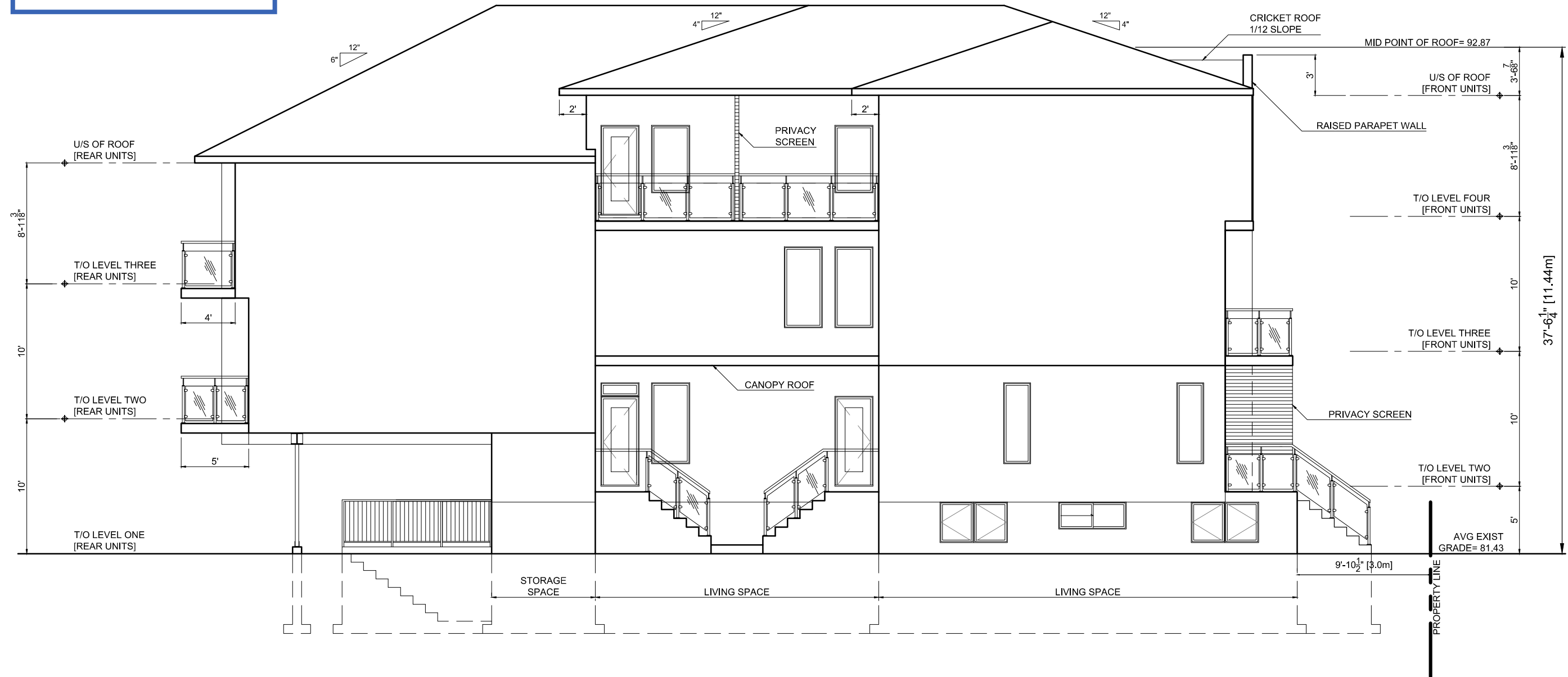
SIDE ELEVATION 2 [WALKWAY SIDE] SCALE: 1/8"=1'-0"
