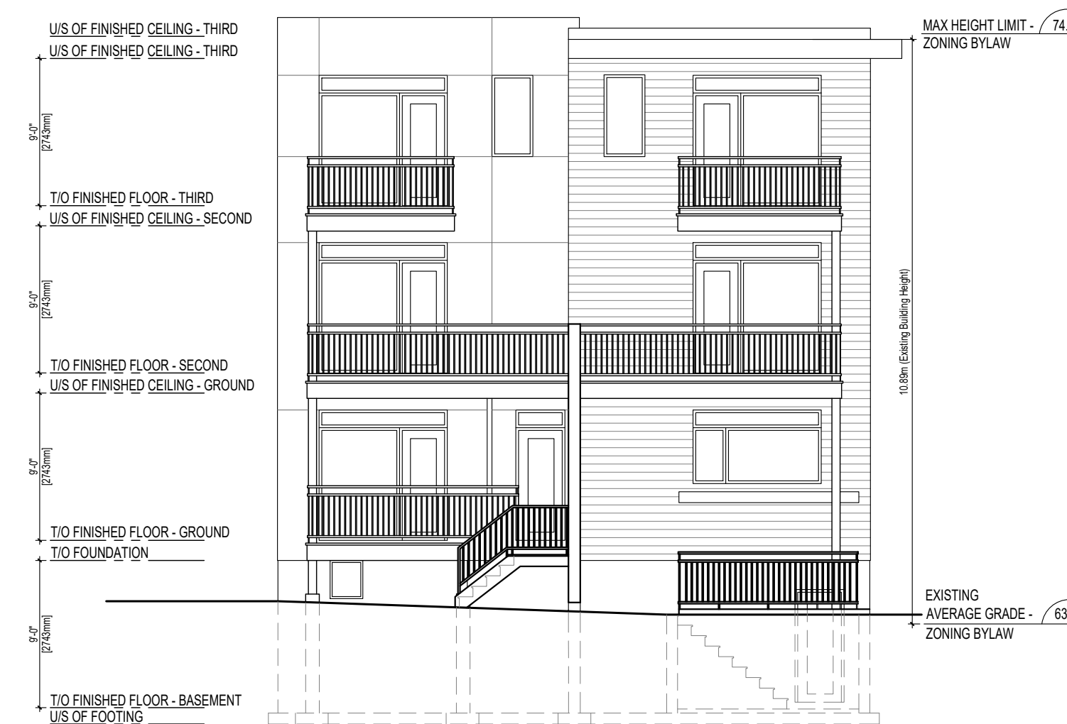
7 PROPOSED SOUTH ELEVATION SCALE: 1 : 100
