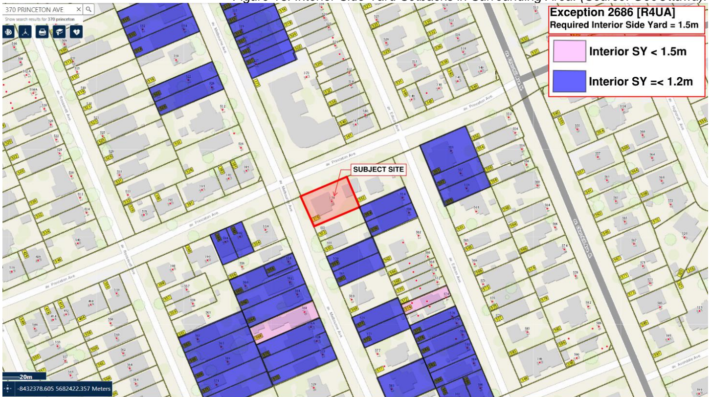
Figure 13: Interior Side Yard Setbacks in Surrounding Area. (Source: GeoOttawa).
