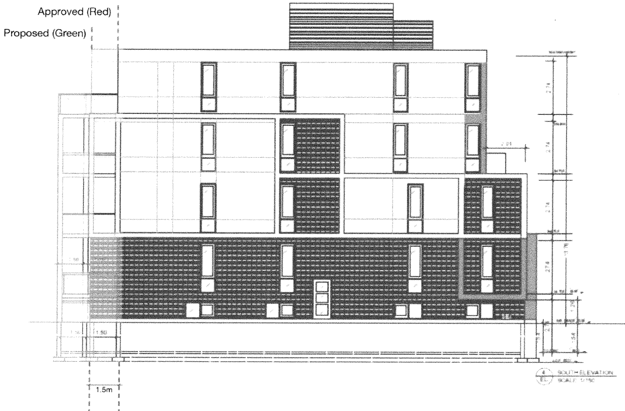
Figure 4: Graphic illustrating the approved and proposed building envelope, with the proposed reduction in the rear-yard setback indicated.
