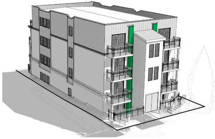
Figure 7: 82 Genest Street as seen from the South. The green highlights indicate proposed thru-wall scupper drains which connect to the building's weeping tile, VADD 2023.
