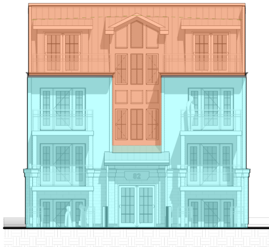
Figure 3: 82 Genest Street: Proposed Front Elevation (Overlaid colour to depict cruciform motif and it’s setbacks from one-another), VADD 2023
