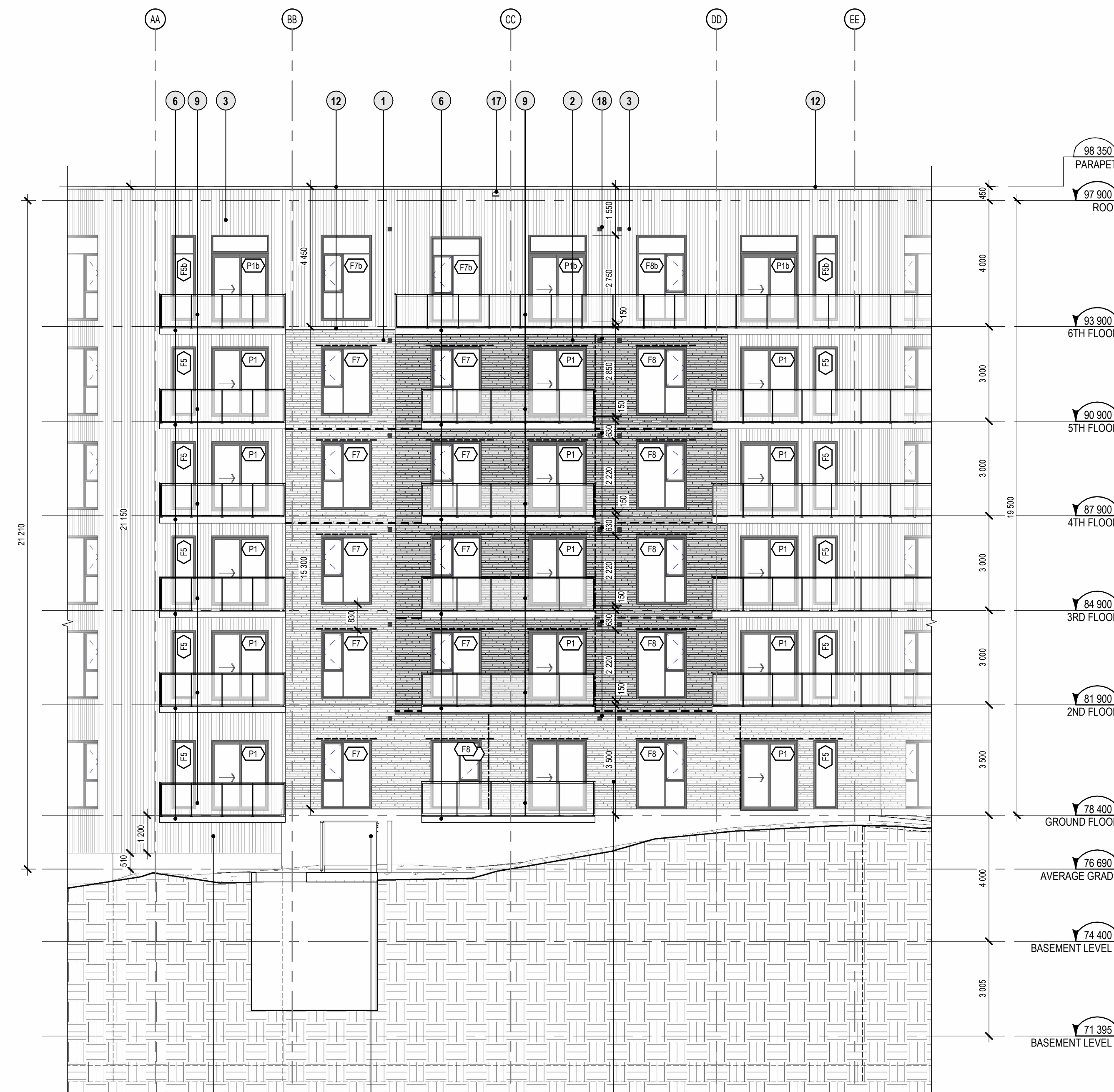
SOUTH-EST CORNER ELEVATION - BUILDING "A" 1:100
