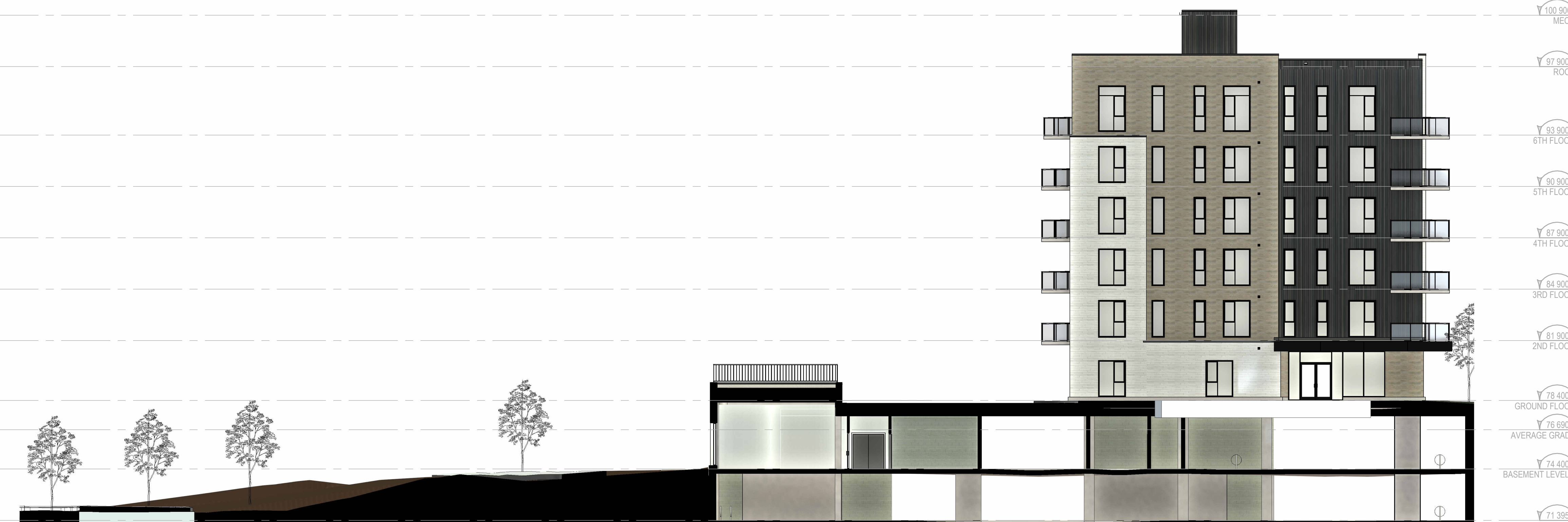
ENTRANCE BUILDING "B" ELEVATION 1:150
