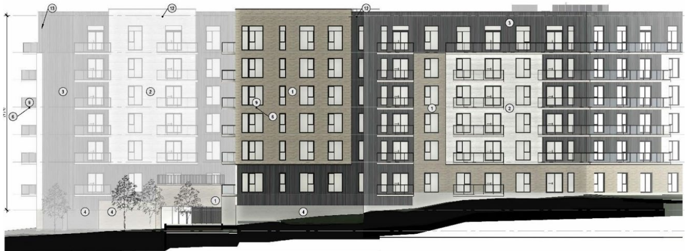
Figure 9: West and Southwest Elevation drawing of the proposed development, showing the change in grade from March Road (right) to Shirley's Brook (left)
