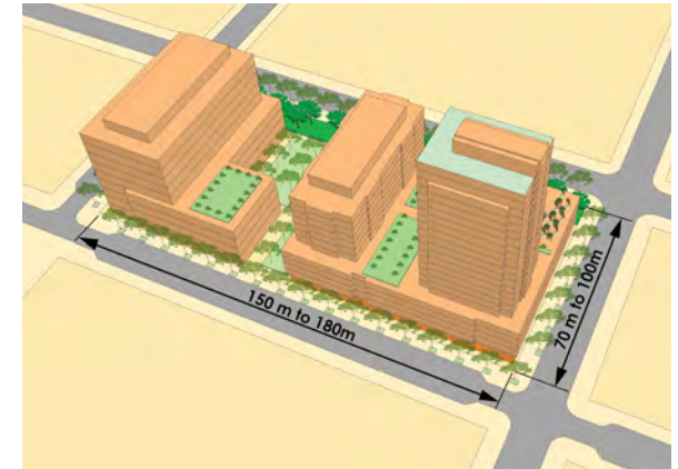
(Figure 4.3) Development on a typical block in the Activity Centres will include high-rise buildings that line active sidewalks with retail, restaurants, or other commercial activity at grade, with other uses located above. Building heights will step down as they transition to lower intensity character areas.
