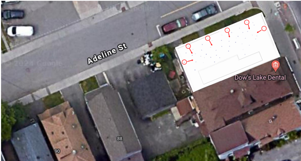
Figure 2.2 – Layout of the location of the six loudspeakers (red circle) and their directionality (red arrow) for 482 Preston Street's patio (imagery obtained via Google Maps)
