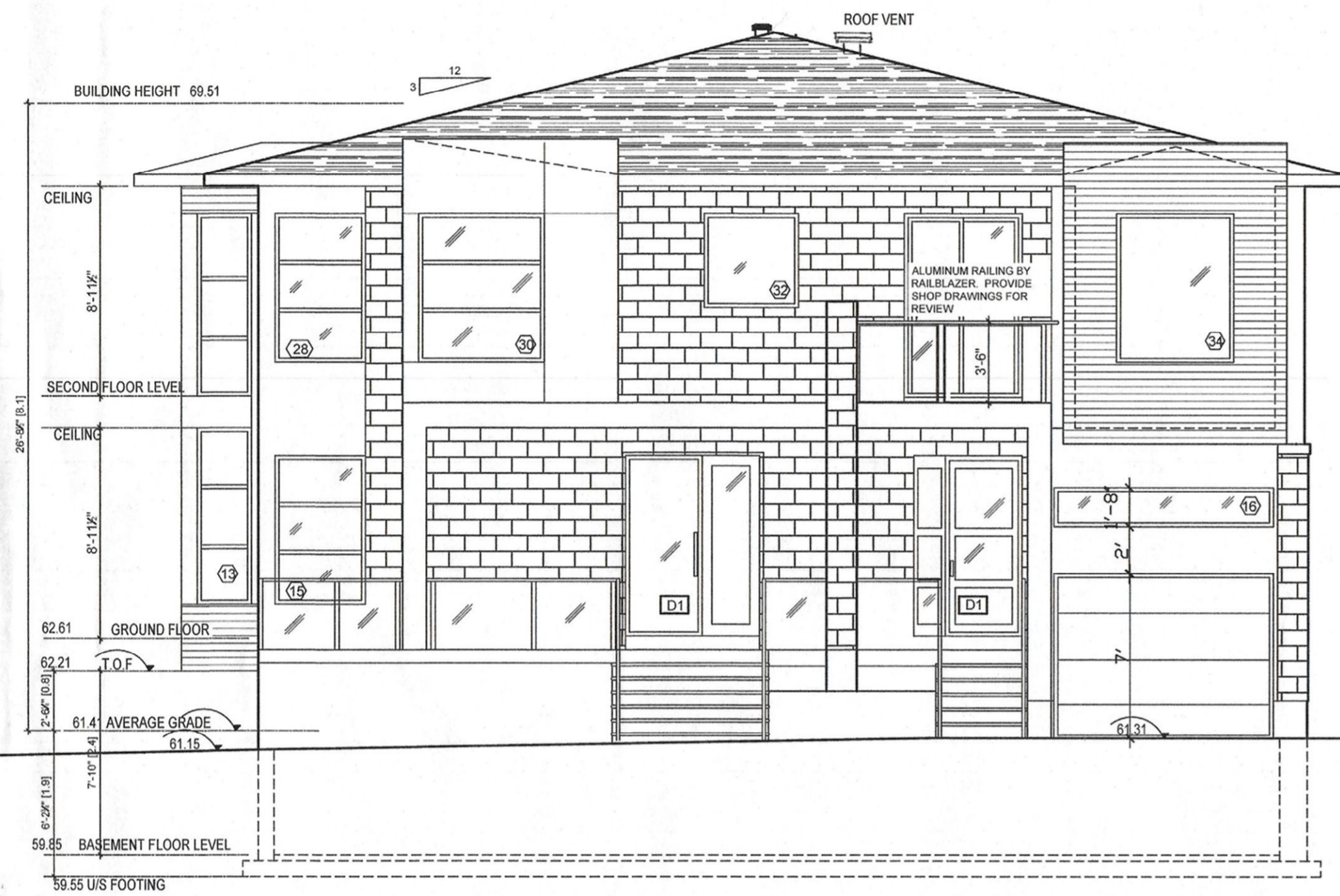
1 SOUTH ELEVATION (FRONT) 3/16"=1'-0"
