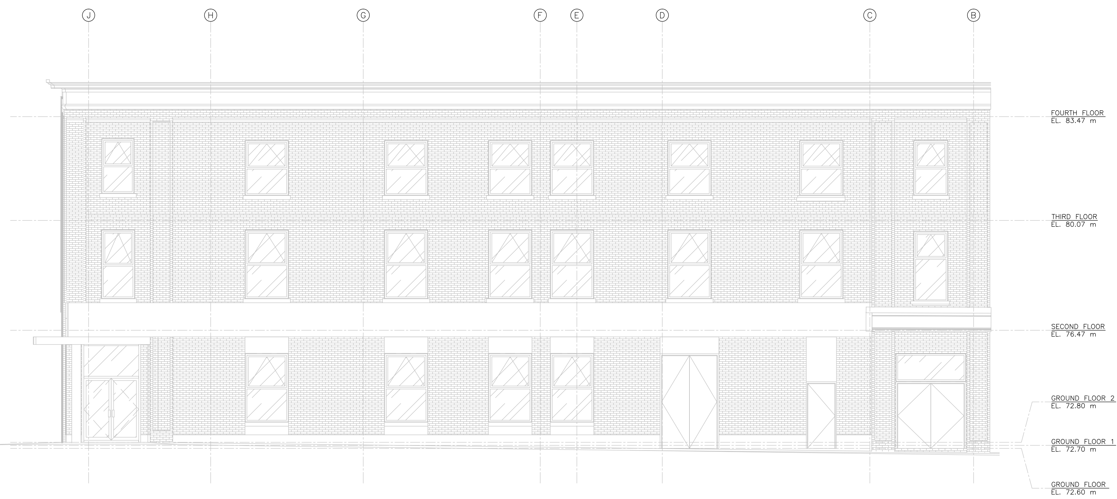
2 NEW SOUTH ELEVATION ZA004 1:75 SHOWN FOR ILLUSTRATION ONLY REFER TO ARCHITECTURAL DRAWING FOR MORE DETAILS
