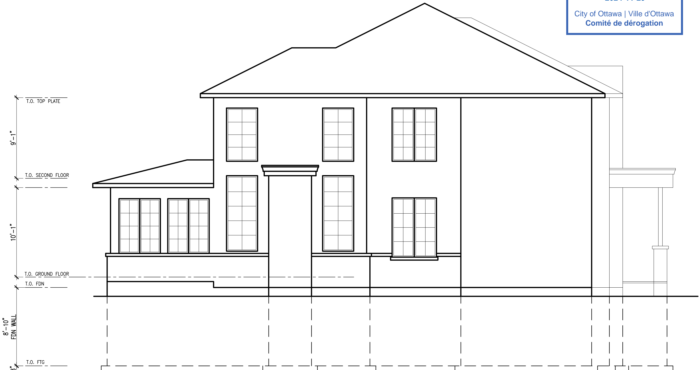
LEFT SIDE ELEVATION - PART 2 SCALE: 3/16" = 1'-0"
