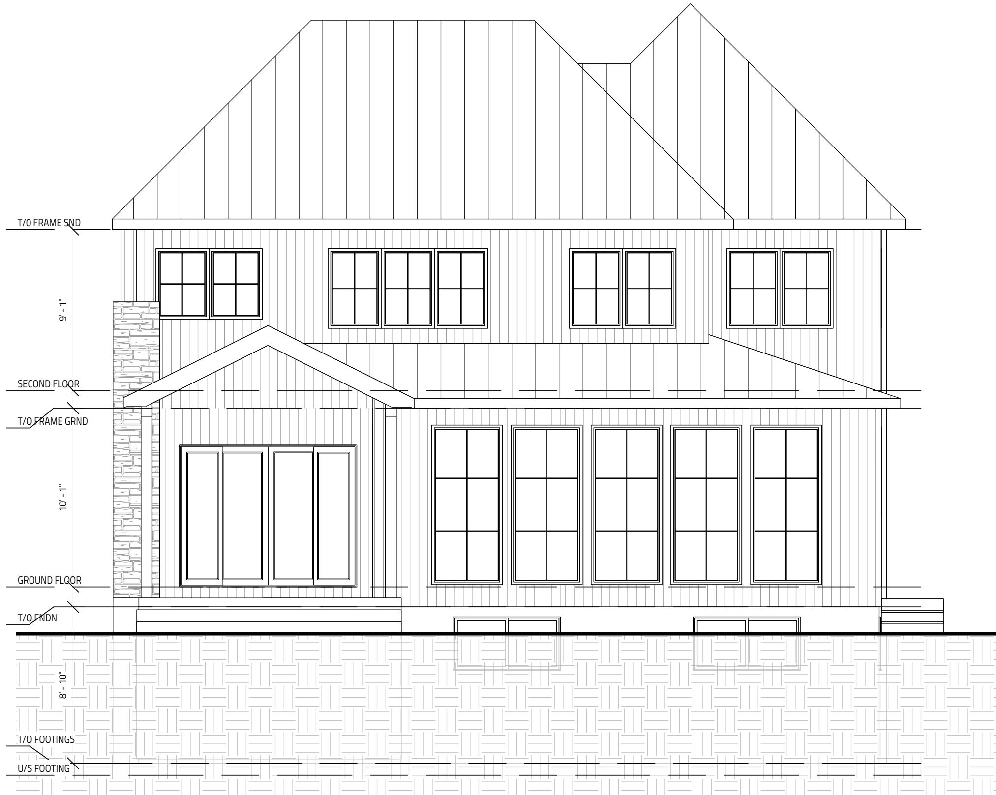
1 REAR ELEVATION SCALE: 3/16" = 1'-0"
