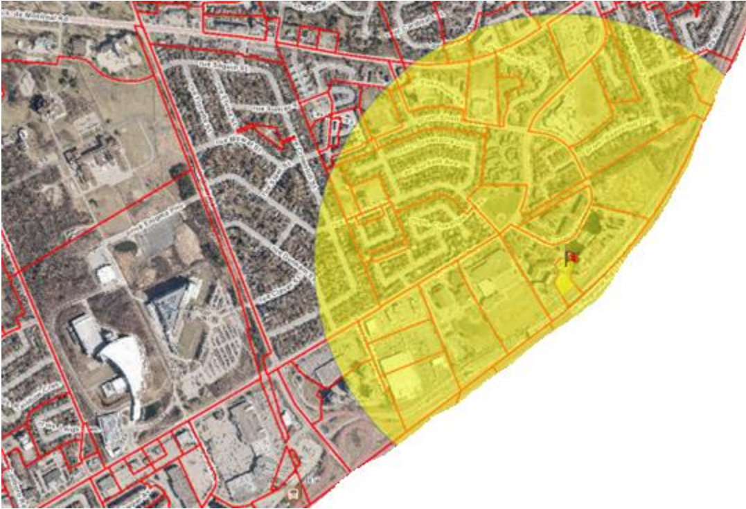
Figure 3: Capture from geoOttawa showing the location of 2040 Arrowsmith Drive and a 900 metres radius. Because Regional Road 174 acts as a barrier to pedestrian movement the area south of the regional road has been removed from the capture. In general, the Official Plan equates a walking time of 15 minutes to be equivalent to a radius of 900 metres or 1,200 metres on the pedestrian network.
