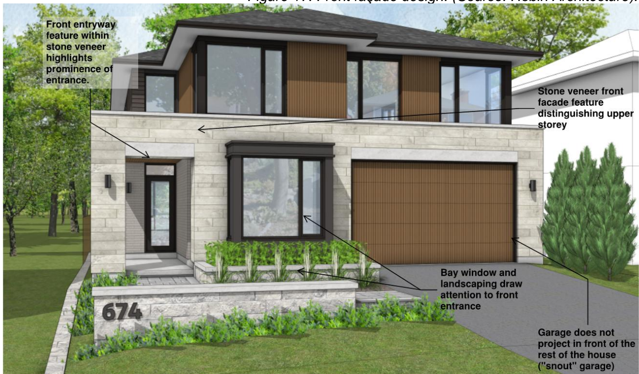
Figure 17: Front façade design. (Source: Hobin Architecture).
