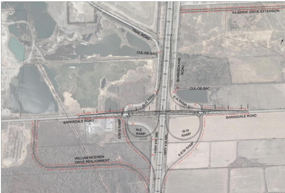
Figure 3b Ultimate Interchange Configuration
