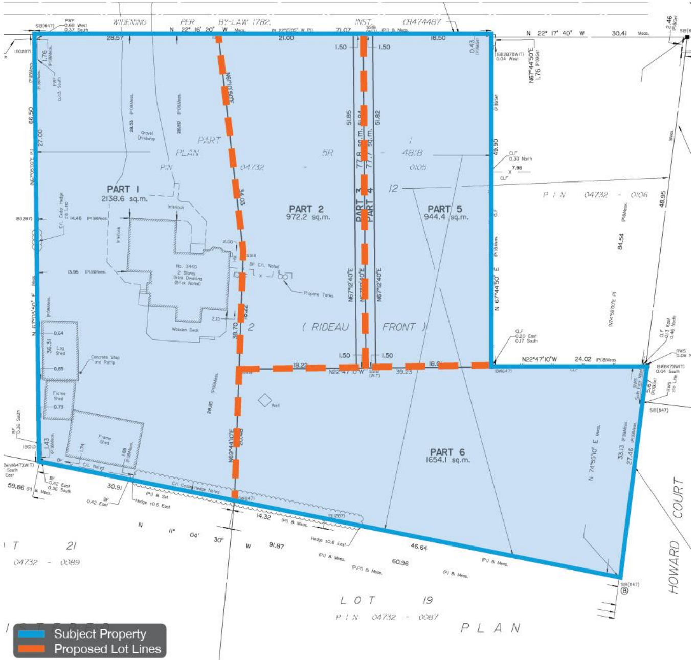
Figure 5: Reference Plan for the subject property with color overlay indicating proposed lot lines.
