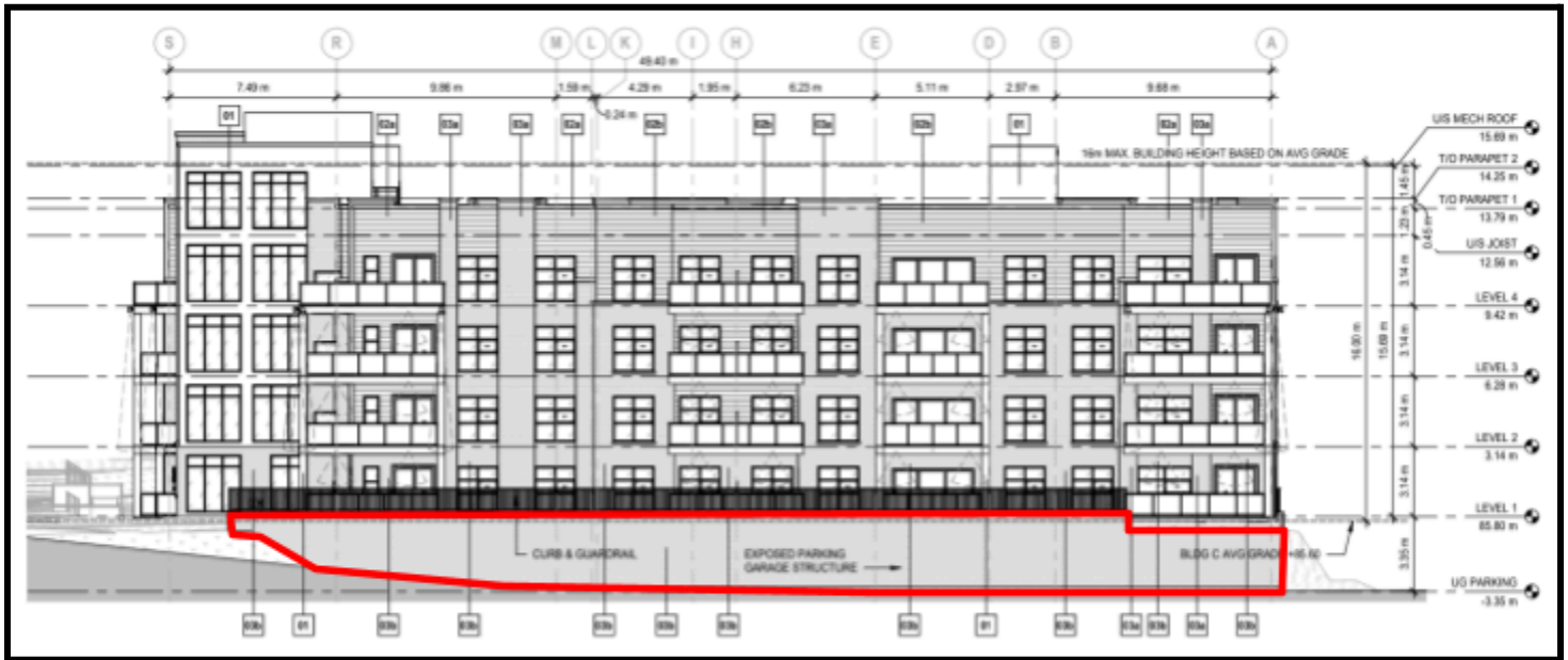
Elevation abutting the northern (rear) lot line (Building C) showing the area of exposed underground parking subject to variance B.
