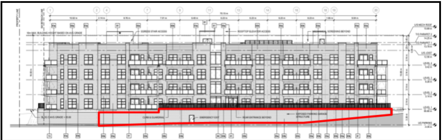
Elevation abutting the western lot line (Building C) showing the area of exposed underground parking subject to variance A.
