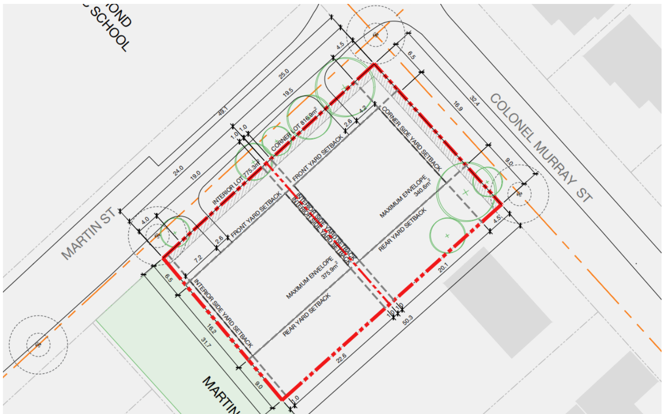
Figure 4: Draft Reference Plan of the subject property, including potential driveway locations showing no conflict with existing trees.
